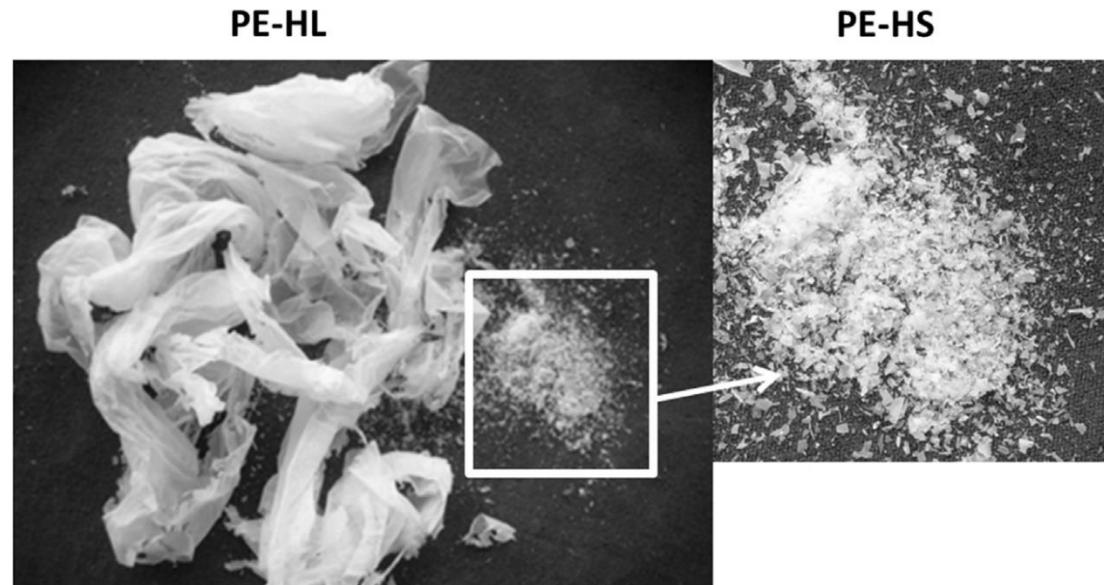
Digital photographs of PE-H after 365 days of incubation in distilled water at 70° C (two fractions: PE-HL – large pieces of investigated material, PE-HS – small pieces of investigated material)
